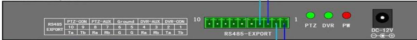
Connect Master Keyboard pin 4 (Ra) with Slave Keyboard pin 2 (Ta)
