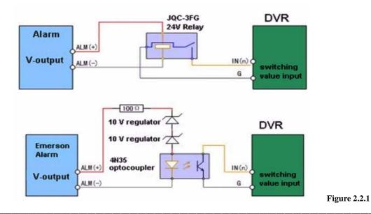
To connect to an AC/DC load, use the following diagram:
