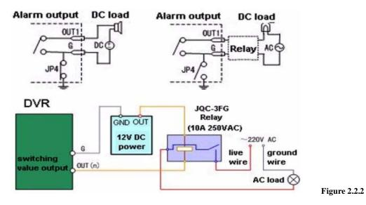
For DC load, JP4 can be used within the limit of 12V/1A safely. If the interface is connected to an AC load, JP4 should be left open. Use an external relay for safety (as shown in the figure above).
