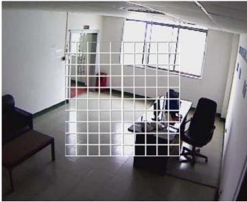
**Figure 9.3. Motion Detection Area**
