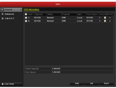
Figure 13.2 HDD Status Changes to Normal
