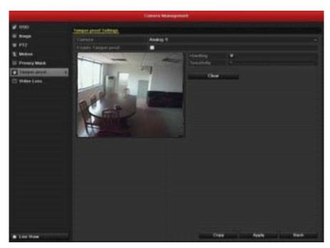
Figure 9.15 Tamper-proof Setup Interface
