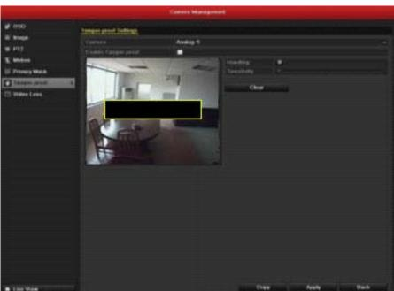
Figure 9+.16 Set Detection Area and Sensitivity of Video Tampering
