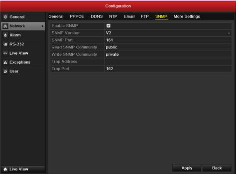
Figure 10.12 SNMP Settings Interface
